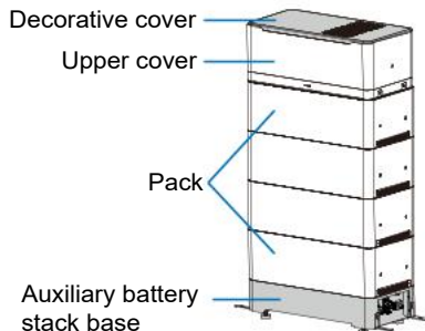
Auxiliary battery stack
