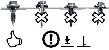
Screw in at a high speed until the drill bit is through the sheeting and then gently tighten at a low speed, using great care or a depth stop. Observe perpendicularity!
