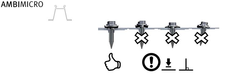
Screw in at a high speed until the drill bit is through the sheeting and then gently tighten at a low speed, using great care or a depth stop. Observe perpendicularity!
