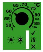
Temperature-adjusting knob 1-6 ... Number of device 13A / 16A ...fuse protection
